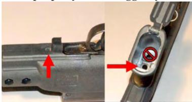
15. Insert the T6 stock tube into the rear of the main body. Use hand pressure to push it in as far as you can, and then gently tap the tube on the back end toward the stock body until it seats flush with the stock body. Use the enclosed screws and nuts to secure the tube into the main stock body.
