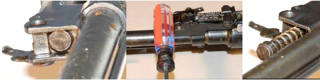
9. If you are replacing the original piston with a new U.S. compliant piston, do so at this time. Your original piston should slide out and the new one will fit in its place.
