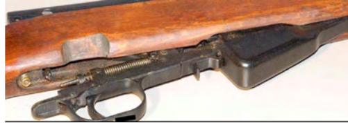
4. The magazine can now be removed by pulling the back of the magazine away from the receiver while pulling the bolt rearward, allowing the front of the magazine to pivot.
